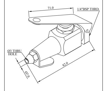
APPLICATION For Blow-off of dirt, dust, oil etc. from shop floor, surfaces, machine working area, deep holes, crevices, geometric patterns, etc. and any hard to reach places.
